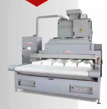
Radio Frequency (RF) is a drying and thermal processing technology based on the dissipation of electromagnetic energy within the product.
