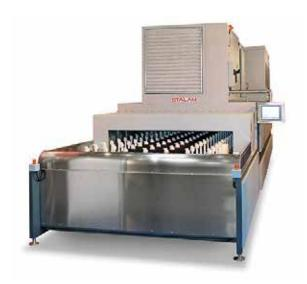
The air forced through the product is heated up to the desired temperature without using any external (additional) energy source by recovering the heat dissipated by the RF generator. Both the RF energy and the warm air forced through the product contribute to water evaporation. This combined process, other than being extremely efficient, enables a precise control of the product's internal temperature, thus optimising the drying quality results.
