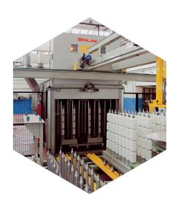
TCRF dryers with 1 or 2 trolleys specifically designed for yarn packages, and a dryer model with 2 trolleys suitable for both tops and packages, are available.
